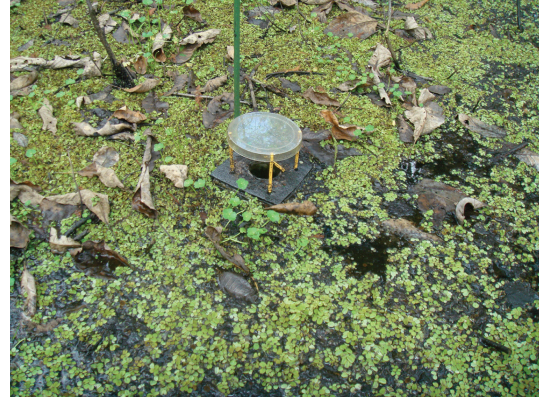
FIGURE 5: Floating pitfall trap shown floating on surface of water in cypress-tupelo-blackgum freshwater swamp.
